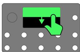
When in The Grid, **swipe down** from the top of the screen to access the I/O Settings menu.
