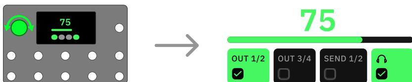
To adjust the Quad Cortex output volume, turn the Master Volume Knob located on the left side of the device.
