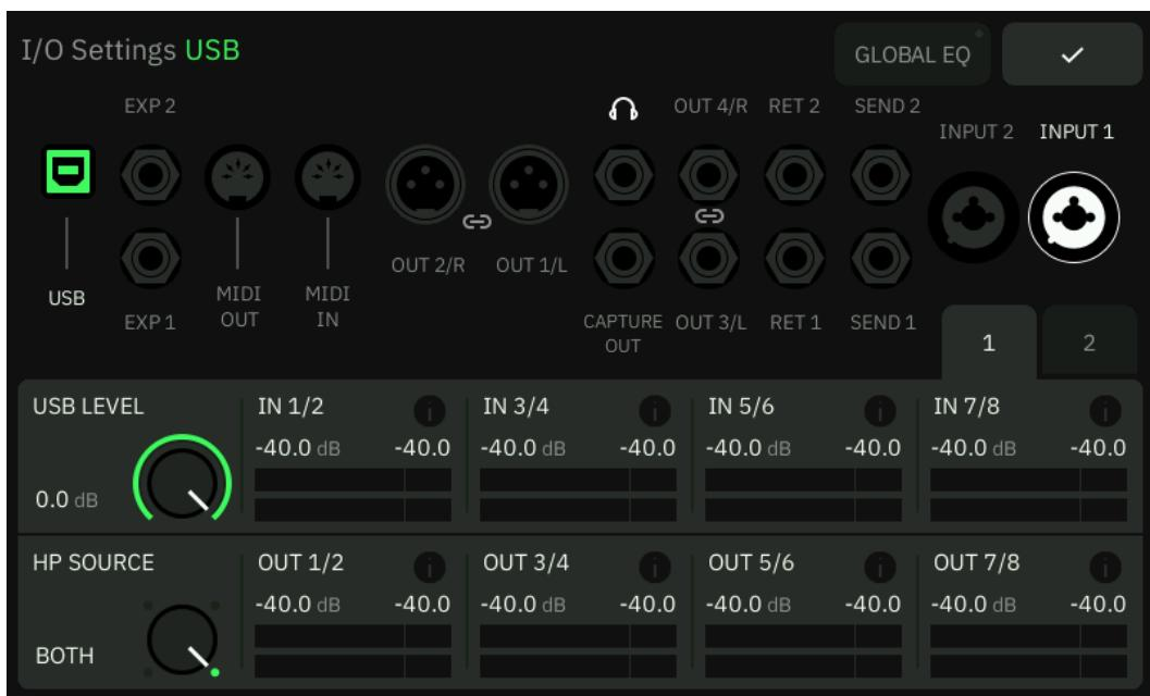
Quad Cortex provides 16 USB audio channels (8 inputs / 8 outputs). These channels are mapped to either host sources or device analog audio ports. **Tap** on a USB or MIDI port to adjust its parameters:
