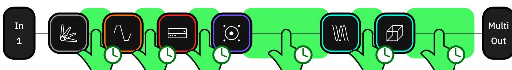
**Tap and hold** any empty slot on the Grid to insert a Splitter or Mixer for the corresponding pair of Rows. Alternatively, dragging any device block from Path A to Path B will automatically create a parallel signal path.
