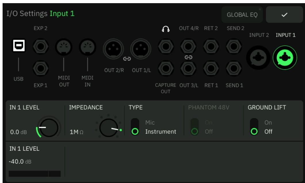
Quad Cortex features multiple audio inputs and outputs. The parameters in the editor panel adapt based on the selected I/O. **Tap** any analog audio port to adjust its parameters:
