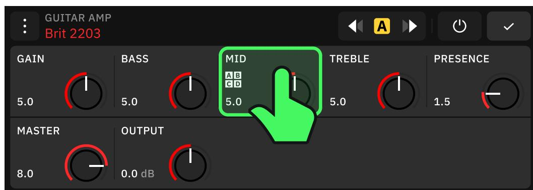
Tap any device block on the Grid to access its parameter editor menu. Then, **tap and hold** a parameter to assign or unassign it to Scenes. Once assigned, the parameter's value will be stored independently for each Scene. This operation can be done in any Mode.
