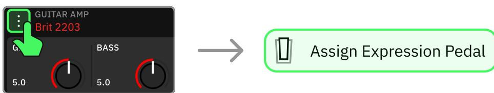
Expression pedals can be assigned to control most adjustable parameters of any block.
