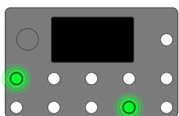
To initiate Recovery Mode, **hold A** and **H** footswitches during the startup screen while booting.
