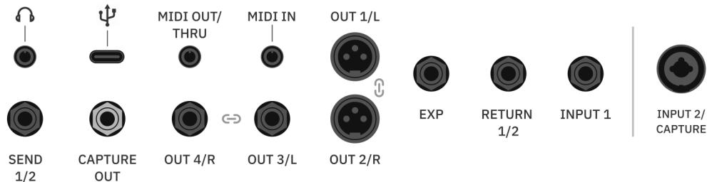
Connect the Quad Cortex mini's **CAPTURE OUT** to the target device's input.
