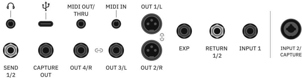
Quad Cortex mini SEND 1/2 and RETURN 1/2 ports use single TRS connectors but can carry two independent signals by splitting the tip and ring connections. This design ensures full compatibility with Quad Cortex content by assigning dual channels to each FX Loop port.
