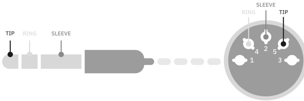
The **TRS MIDI Type-A** connection is the official standard adopted by the MIDI Association. The Quad Cortex mini MIDI ports will be compatible with any TRS MIDI cable that meets the following wiring requirements:
