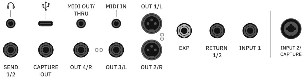
Connect the expression pedal to the Quad Cortex mini **EXP** input using a **TRS cable**.
