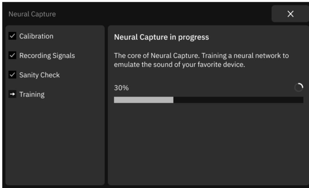
During the Neural Capture Version 1 process, the Quad Cortex mini measures the latency of the target device and sends a series of recorded test signals through it. These signals are then analyzed to model the device's sonic characteristics. After a brief sanity check, the Quad Cortex mini trains a neural network to accurately replicate the tone and dynamic response of the target device.
