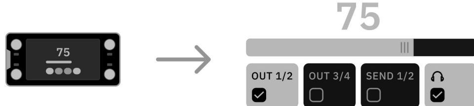
To adjust the Quad Cortex mini output volume, use the **+** and **-** buttons located on the left edge of the device.
