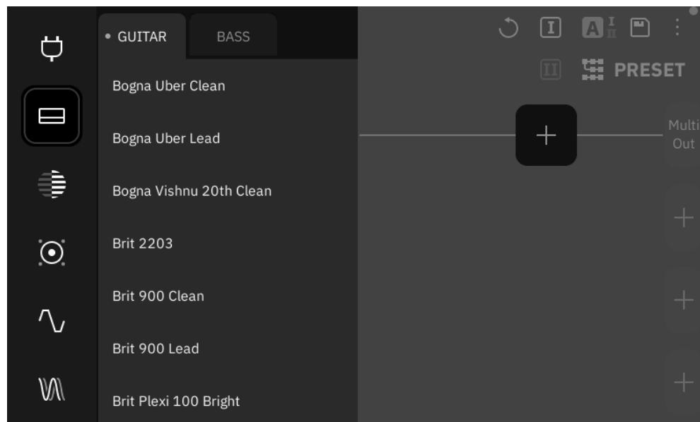
The Virtual Device List provides access to all virtual devices available that can be placed on The Grid. It allows you to browse by category, search for specific devices, and manage your favorites for quicker access.
