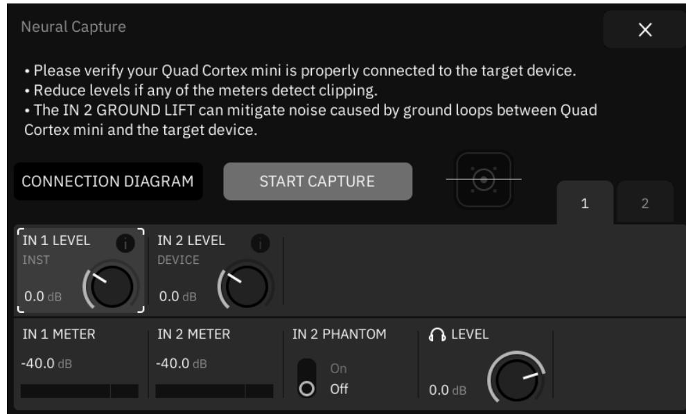
Before starting the Neural Capture process, ensure the microphone position and target device settings are adjusted to your preference. Reduce input levels if any meters indicate clipping.
