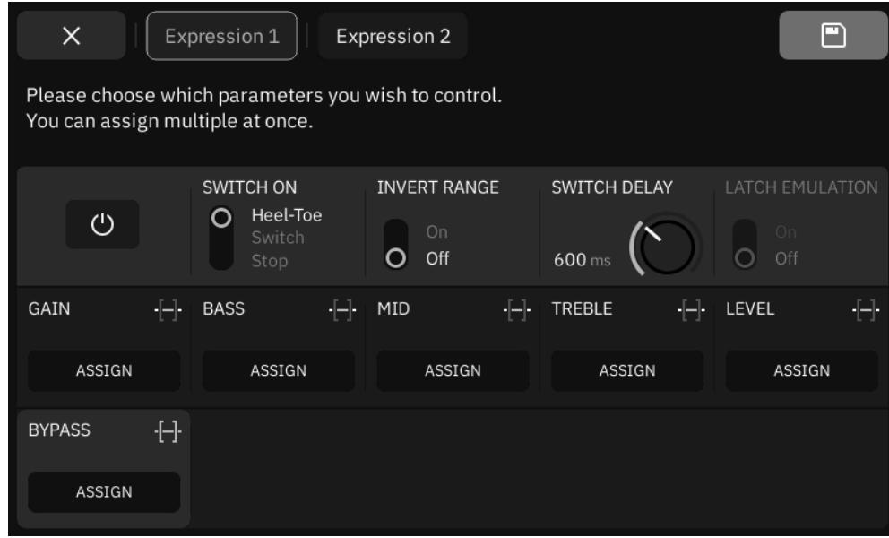
Blocks can be engaged or bypassed using expression pedals. To configure this, first assign an expression pedal to a device block by opening its contextual menu and selecting **Assign Expression Pedal**. Then, tap **ASSIGN** under the **BYPASS** parameter to access additional options:
