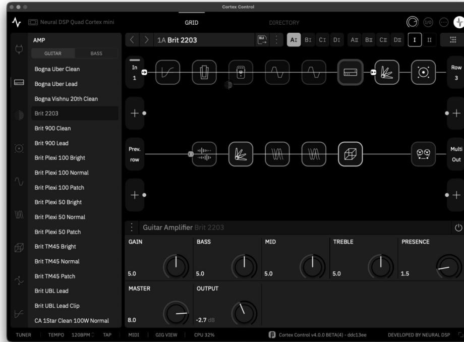
Cortex Control features an intuitive and **expanded version of The Grid**, giving you a clear overview of the current active Preset. The Grid displays your virtual devices, signal routing, parameter values, active Scene, Tempo, and CPU usage.
