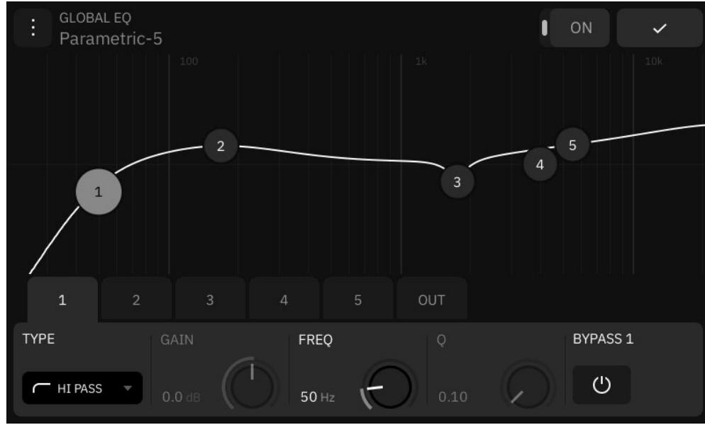
The I/O Settings menu includes a 5-Band Parametric EQ that can be assigned to one or both output pairs.
