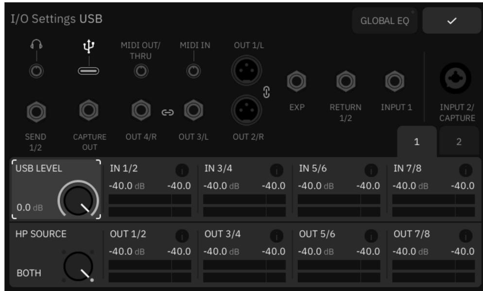
Quad Cortex mini provides 16 USB audio channels (8 inputs / 8 outputs). These channels are mapped to either host sources or device analog audio ports. **Tap** on a USB or MIDI port to adjust its parameters:
