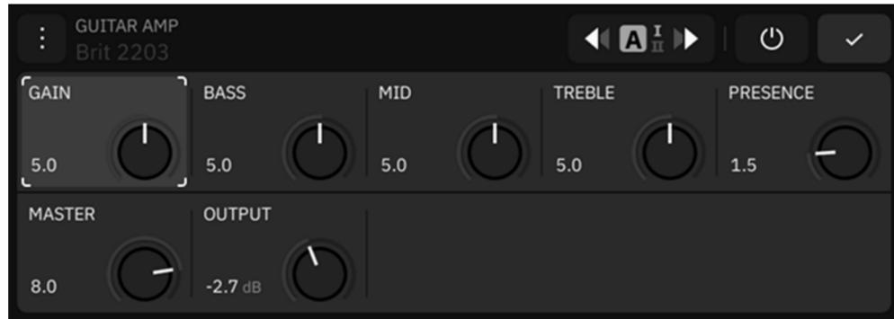
The layout of a parameter editor depends on the selected block. For most devices—including splitters, mixers, and I/O blocks—the editor occupies the bottom half of the screen. Certain devices, such as Cabs, Looper X, and other special blocks, utilize a full-screen layout to provide additional controls and options.
