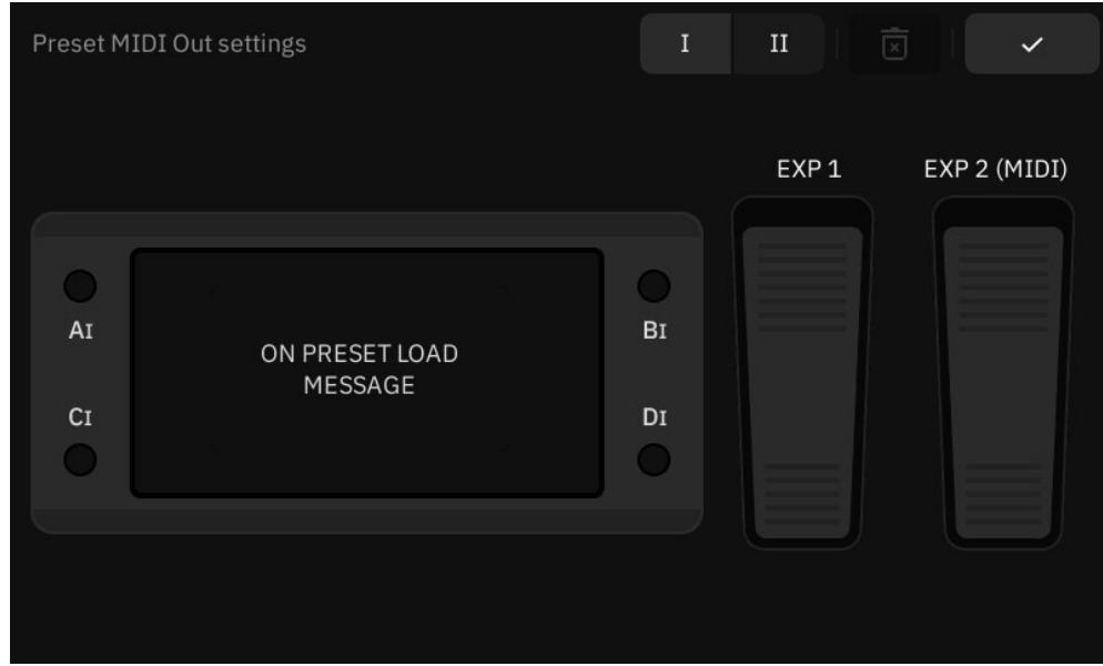
You can assign up to **12 MIDI messages per footswitch** that will be sent via USB and/or TRS MIDI simultaneously upon pressing a designated footswitch. Different MIDI messages can be assigned to Footswitch Pages I and II.
